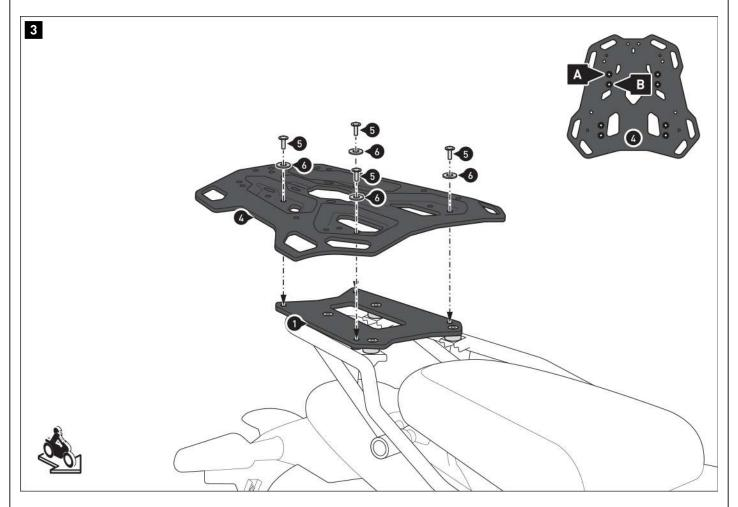
$\triangle$  **NOTE:** Depending on the space available, screw the luggage carrier (4) to the marked attachment position (A) or (B) as shown in the detailed drawing.
