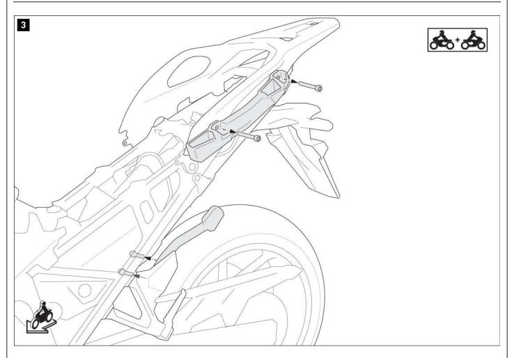
Loosen the indicated screws of the original side carrier and remove the parts  ${\it from\ both\ sides}$  of the vehicle.
