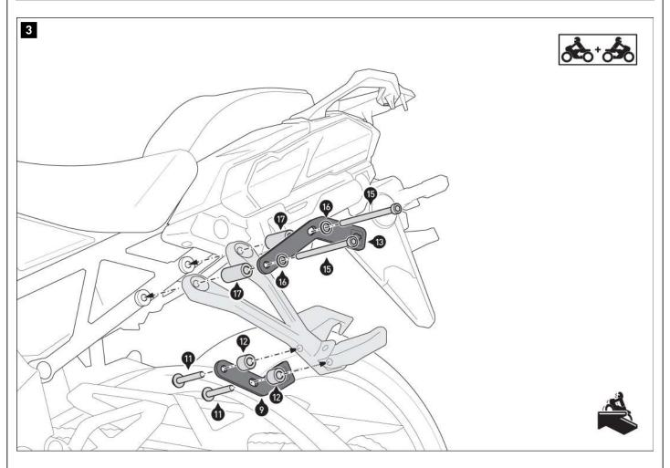
Screw the fastening tabs [9/10] onto both sides of the pillion footrest holders.  $\triangle$  WARNING: Use a liquid threadlocker! Do not tighten the screws [11] yet.
