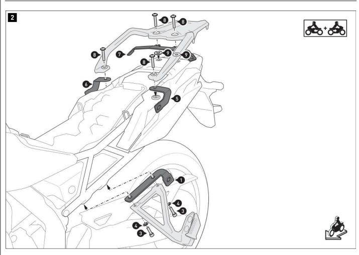
Screw the fastenings straps (1), (2), (5) and (6) as well as the crossbar (7) to both sides of the vehicle. **A WARNING: Use a liquid threadlocker!** Do not tighten the screws yet.
