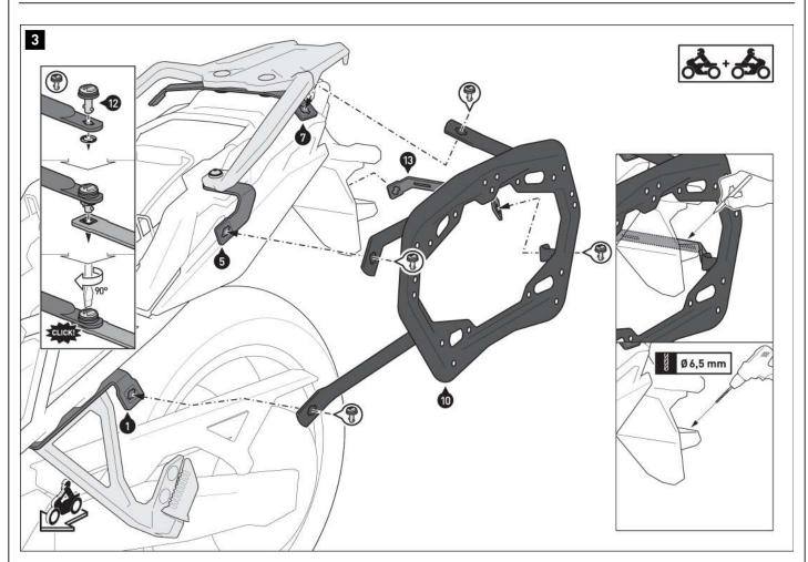
Connect the side carriers (10) and (11) to the fastening straps (1), (2), (5) and (6) and crossbars (7) and (13) using the quick-release fasteners (12). Secure the quick-release fasteners using the lock washers. Use a sharp object (for example, a screwdriver) to mark the drilling position on the outside of the license plate holder. Dismantle the side carriers (10) and (11) together with the crossbar (13).
