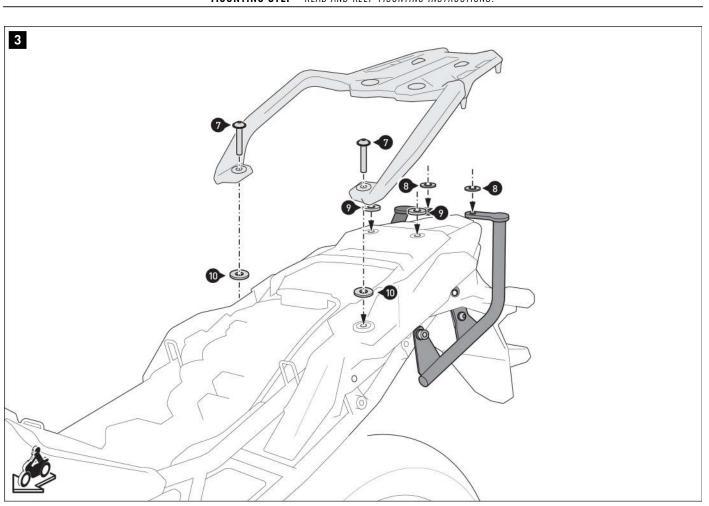
▲ **NOTE:** When connecting to the SW-MOTECH side carrier, spacers (9) and (10) are no longer required. In their place, mount the side carrier using the parts from the rack.
