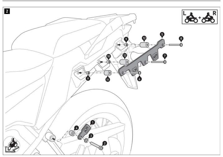
Screw the mounting brackets (1) onto both sides of the passenger footrest
