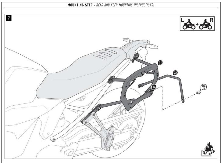
Use the the quick-release fasteners (13) to connect the crossbar (22) on both sides to the fastening tabs (14).
