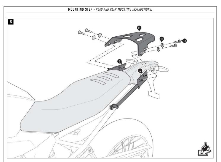
Screw the rack (11) onto the mounting struts (4) and (5). **A WARNING: Use liquid threadlocker!** When the rack (11) has been loosely attached, tighten the screws (12) as described in the mounting instructions.
