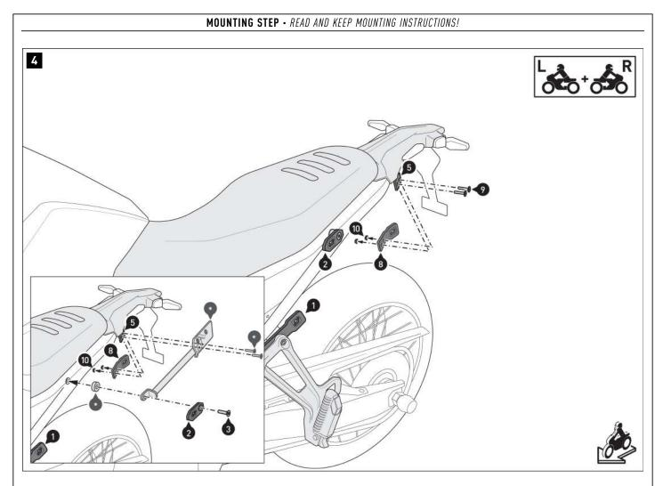
▲ **NOTE:** If you are also installing the SW-MOTECH luggage rack (\*), screw the parts together as shown in the detailed drawing. The spacers (4) and screws (9) are not required in that case. Instead, use the spacers (\*) and screws (\*) included with the luggage rack.
