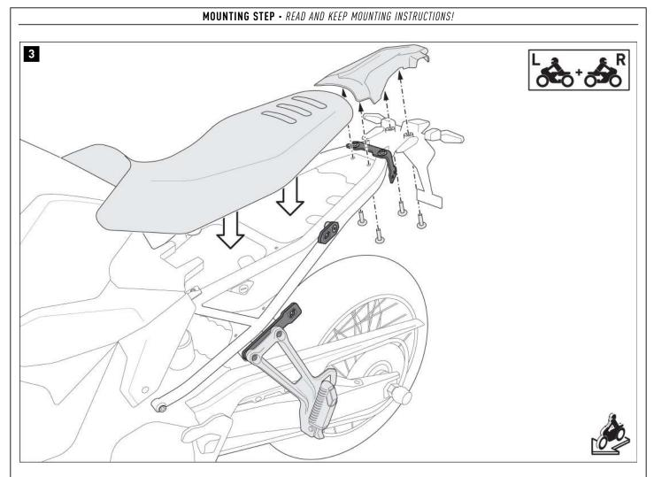
Install the rear cover. Tighten the original screws according to the manufacturer's instructions.
