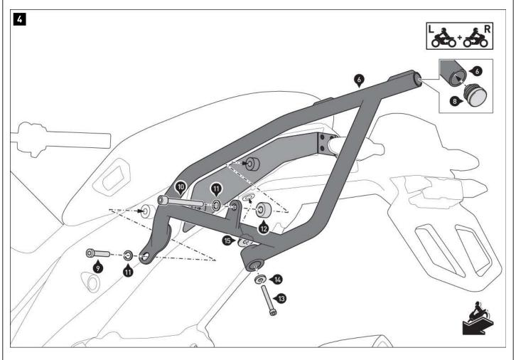
Press the plastic plugs (8) into the ends of the mounting struts (6/7).
