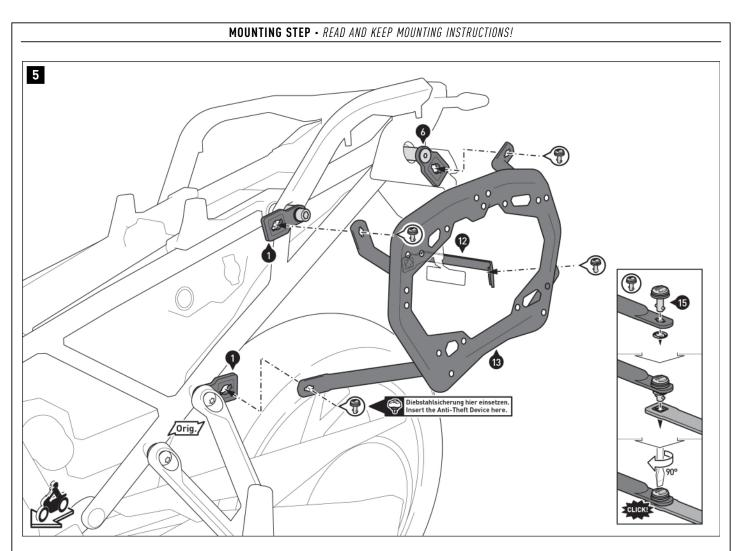
$\triangle$  **NOTE:** The SW-MOTECH anti-theft protection devices are available separately; mount the anti-theft protection devices on both sides at the marked position.
