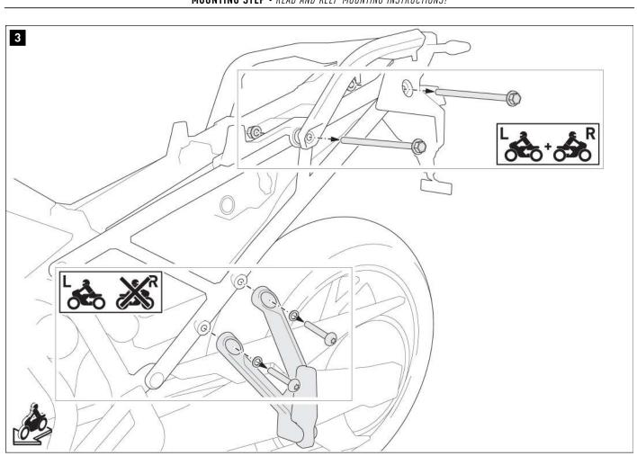
Remove the screws and nuts (as shown in drawing) from both sides of the rear of the vehicle. Then remove the passenger footrest from the left side of the vehicle.
