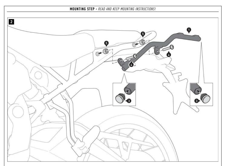
Insert the plastic plugs (3) into the ends of mounting struts (1) and (2).
