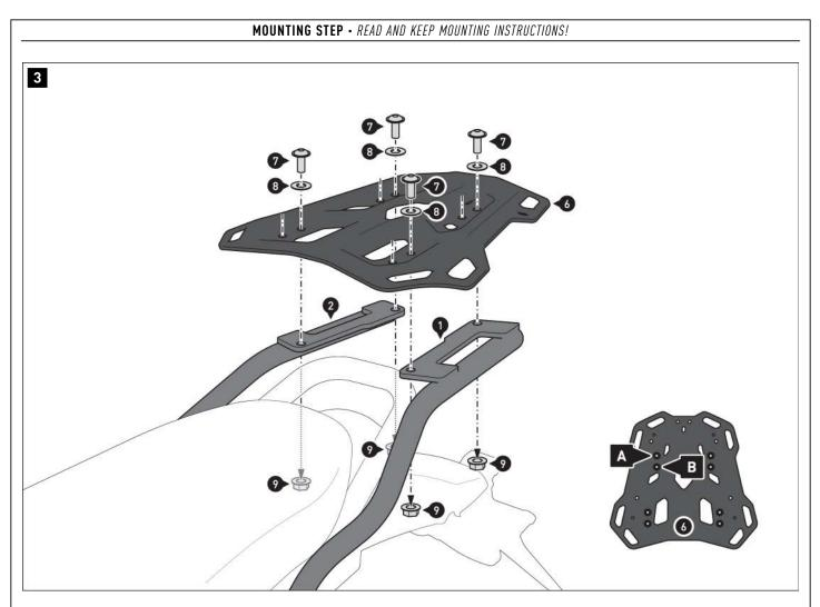
$\triangle$  **NOTE:** Depending on the space available, bolt the rack to mounting position (A) or (B), as indicated in the detailed drawing.
