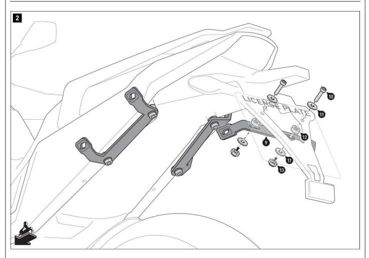
Screw the crossbar (9) to your number plate on the license plate holder. Do not tighten the screws yet.
