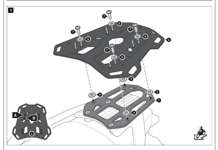
$\triangle$  **NOTE:** Depending on the space available, bolt the rack to mounting position (A) or (B), as indicated in the detailed drawing.
