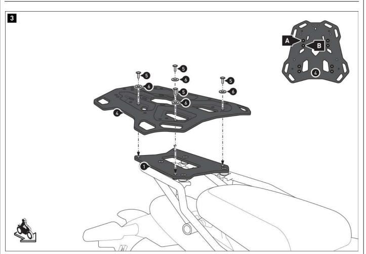
▲ **NOTE:** Depending on the space available, screw the luggage carrier (4) to the marked attachment position (A) or (B) as shown in the detailed drawing.
